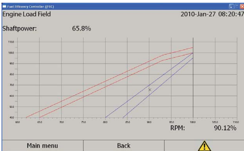
▲ Meaningful graphics allow the operation at the ideal engine operating point and thus the optimization of fuel consumption: Display of the shaft power as a function of engine speed.
